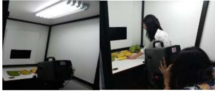
Figure 3. Color inspection with spectrometer color measurement
