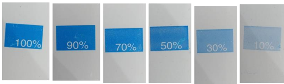
Figure 2. Printed samples of dot area on PP white film
